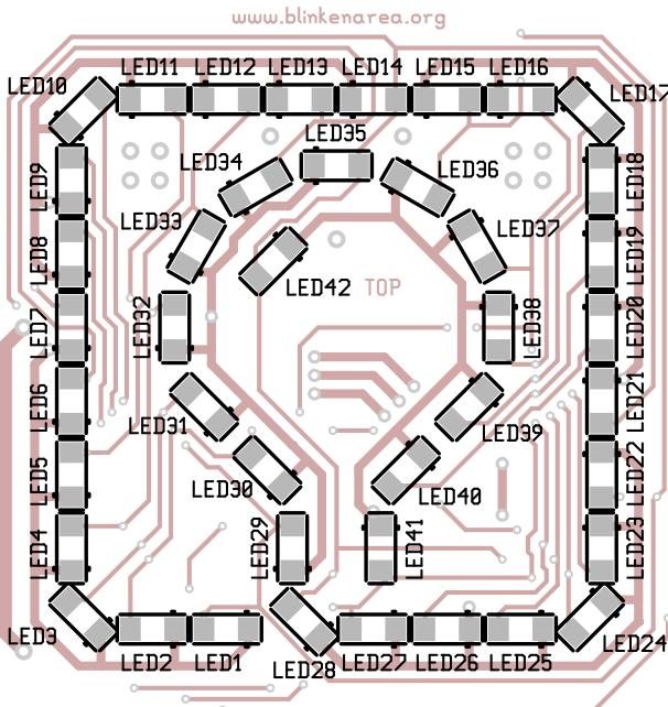
The schematic drawing of the board shows to what positions and in which orientation the parts have to be soldered.
